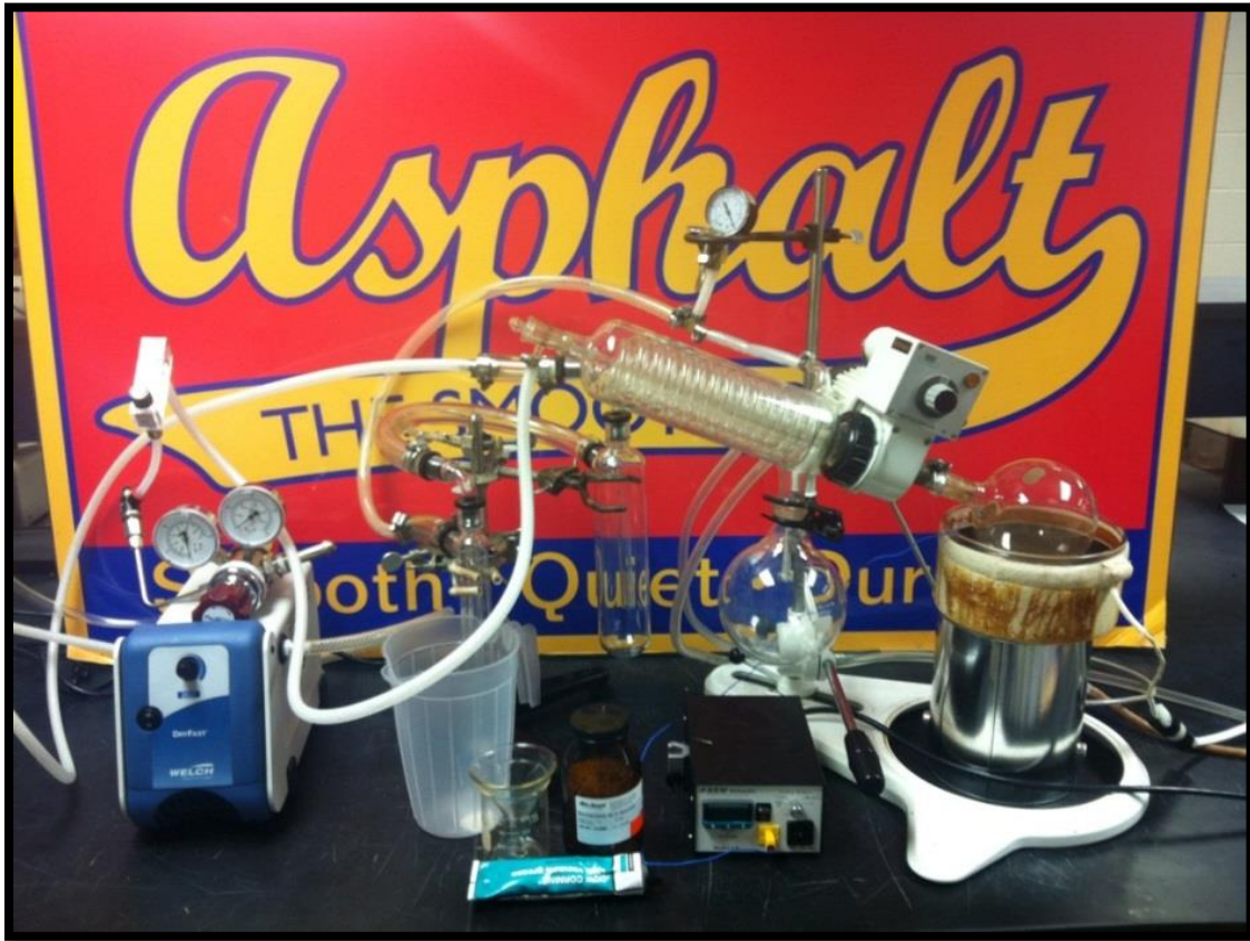
Figure 3.12 Rotary evaporator binder recovery system (Photo courtesy of Sheng Tang)
